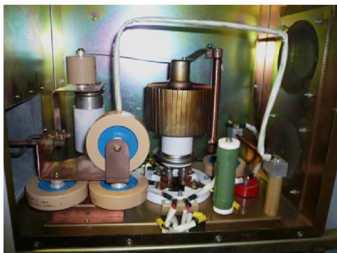
Advanced 2.5 kW HF Generator with ceramic tube (3.5 kW rating), grid & plate current monitoring
