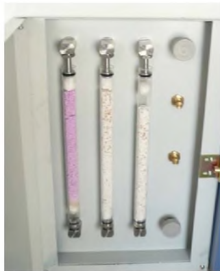
Easy accessible reagent tubes and flow/pressure adjustment
