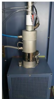
Heated dust filter & furnace head
